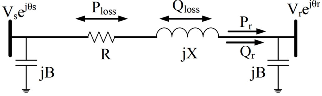
Figure 1. The equivalent circuit of an AC line
